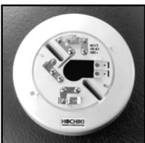
The NS6-100 is a 6" diameter base that has no current limiting nor annunciation output features. A direct short occurs across the loop when the detector is actuated. Heat detectors are not recognized as proper detection for life safety protection, therefore they should be utilized only for the protection of property.
