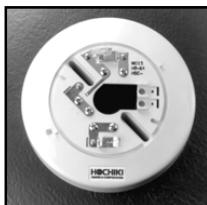
The HSC-(XXX)L Series is a 6" base featuring a current limiting resistor, latching annunciation output and a latching circuit so the alarm LED will remain lit until the control panel has been reset. Heat detectors are not recognized as proper detection for life safety protection, therefore they should be utilized only for the protection of property.
